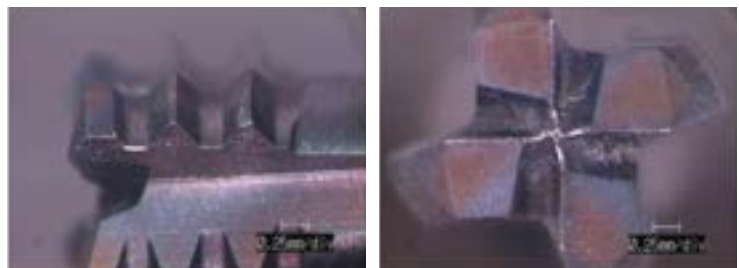
Epoch D Thread Mill after threading 400 holes.
