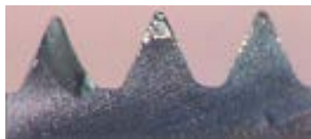
Conventional after threading 10 holes.
