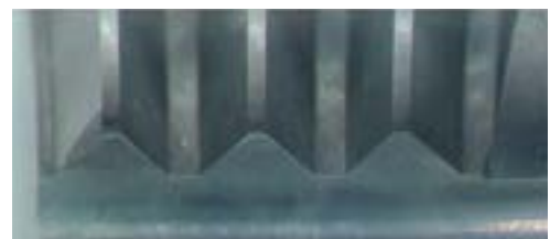
Epoch Thread Mill after threading 300 holes.
