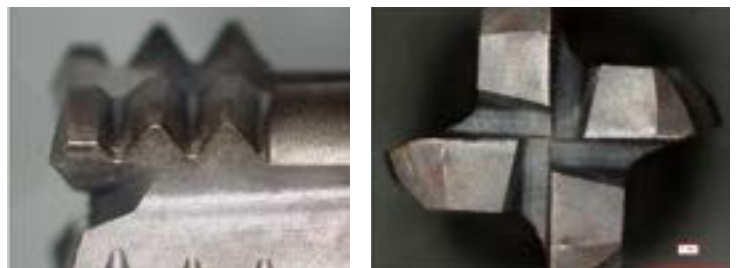
Epoch D Thread Mill after threading 50 holes.
