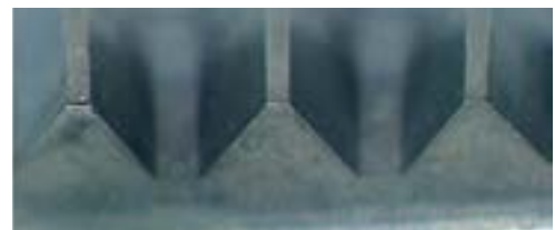
Epoch Thread Mill after threading 300 holes.
