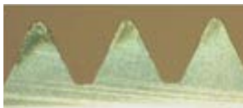
Epoch Thread Mill after threading 50 holes
