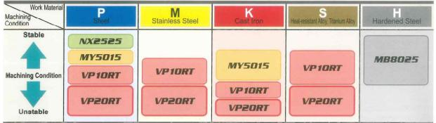
Note1) VP20RT is the first recommended grade for materials other than hardened steel. Note2) For VP10RT, VP20RT and MY5015, wet cutting is recommended.
