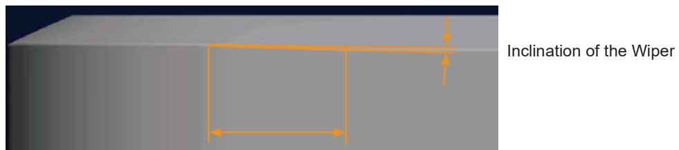
The Optimum Wiper Width Applying slight slope on the wiper cutting edge reduces cutting resistance.
