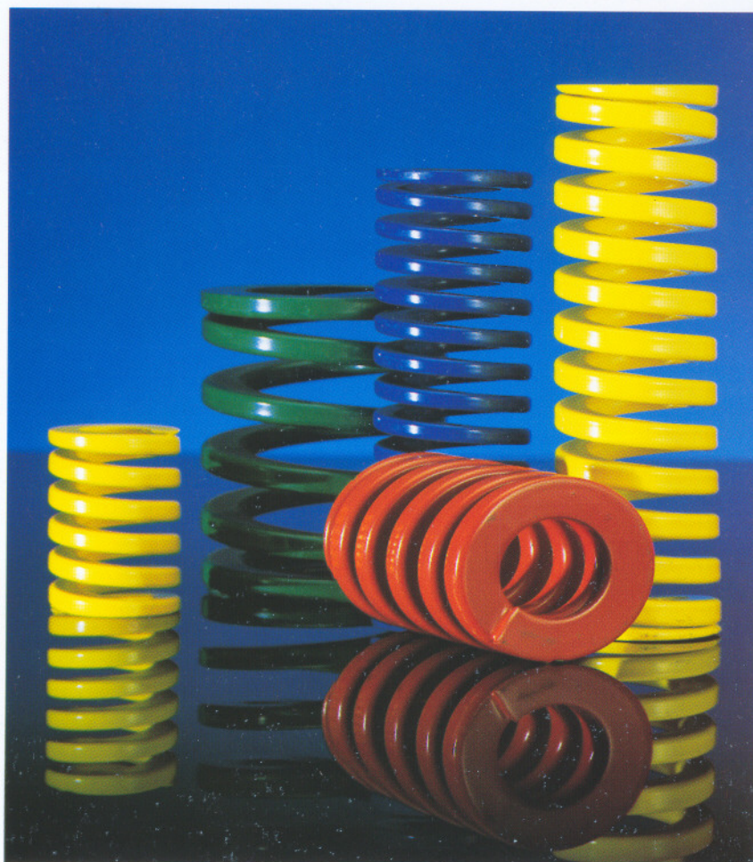
Ends of each spring are closed and ground square to assure every spring will stand on either end, providing a maximum bearing surface and improving performance.
